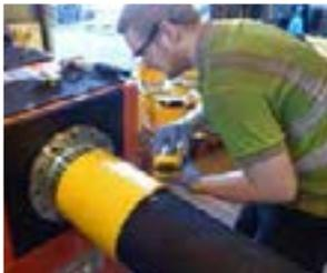
**316L Stainless Steel fittings** can be internally swaged, leaving no potential 'bug-traps' in the bore of the hose. **Perfect for hygienic applications.**
